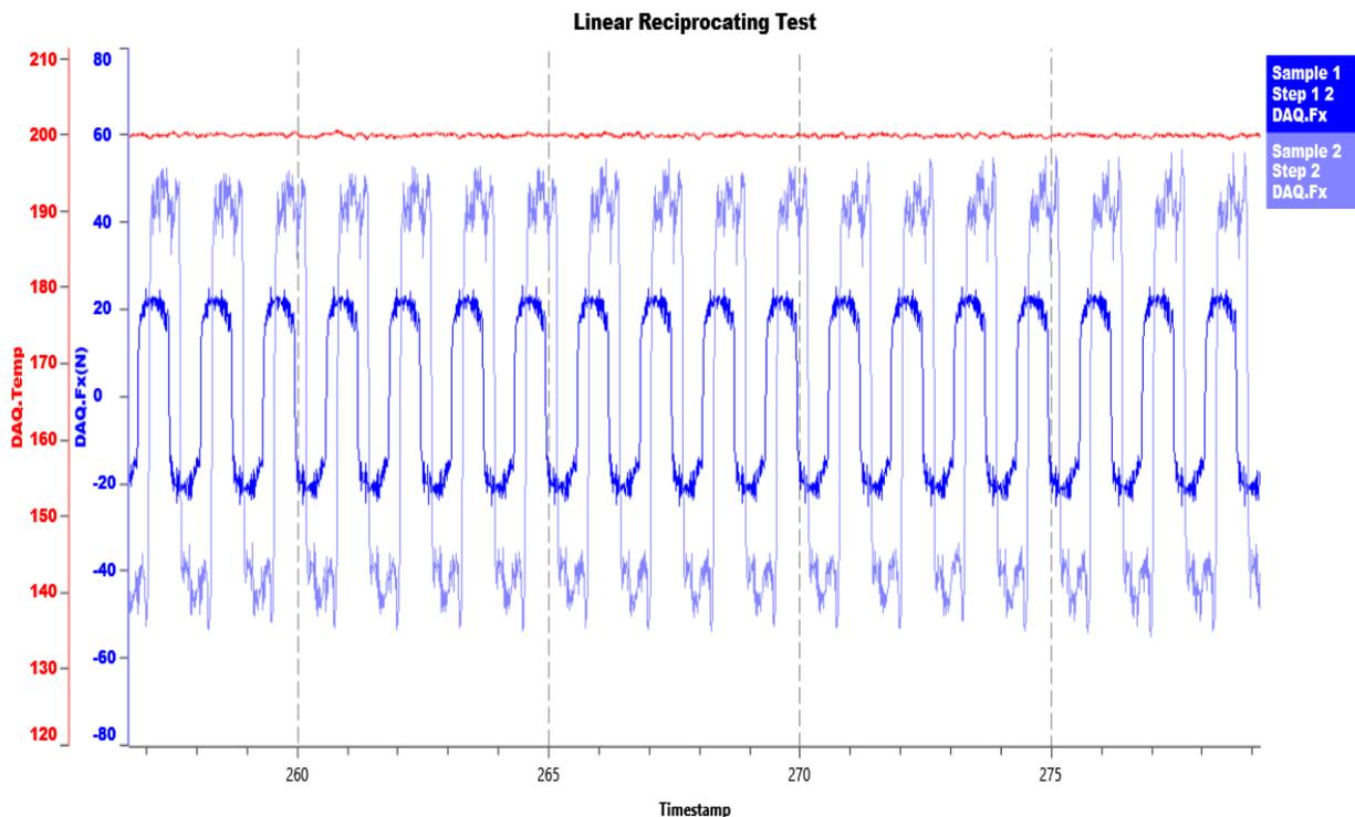
Figure 4: Data showing comparison of two different samples tested at 200C, 200N in Linear Reciprocating Test
