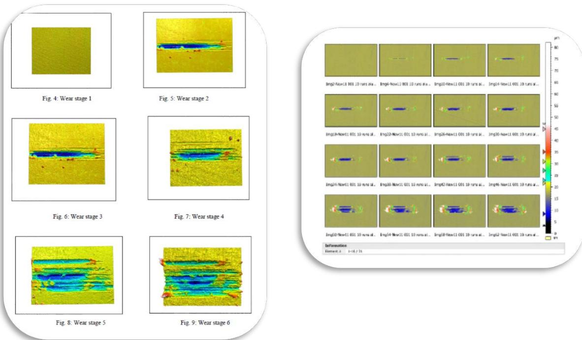
Figure 5: Wear vs time for linear reciprocating test. Every 10 minutes the sample was moved from mechanical testing area to the 3D Profilometer to characterize the progress of wear vs. time.
