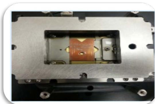
Figure 2: Liquid container for linear reciprocating test
